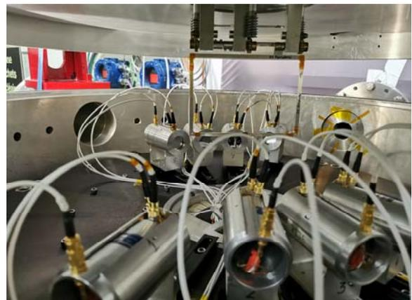
Figure 1: The inner view of the Medley chamber, showing the eight telescopes for detection of secondary light ions. The rectangular frame, attached to the lid of the chamber, is holding a circular  $\text{CH}_2$  target, supported by thin wires.
