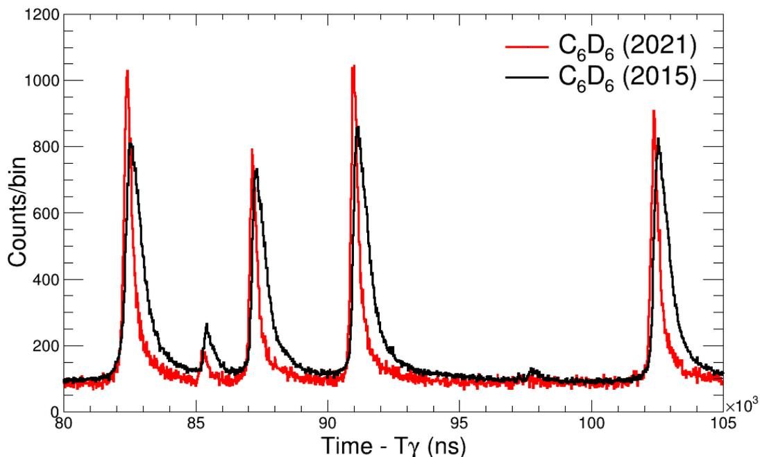
Fig. 1.- Time-of-flight spectrum of  $^{197}\text{Au}(n,\gamma)$  measured with  $\text{C}_6\text{D}_6$  detectors at n\_TOF-EAR2 (measuring position at 19.5 m) with the previous (2015) and the upgraded (2021) spallation target. The neutron energy between 200 and 300 eV is displayed.
