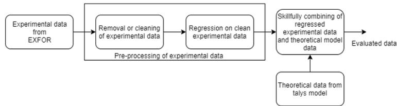
Fig. 1: Block diagram for evaluation of nuclear data
