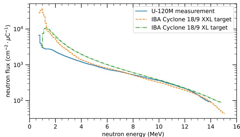
Fig. 2: Comparison of neutron spectra in 1 m from the target in straight direction for different target assemblies
