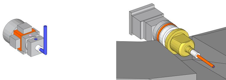
Fig. 1: Comparison of target assemblies at the cyclotron U-120 M at NPI (left) and at the cyclotron IBA Cyclone 18/9 at UJV (right)
