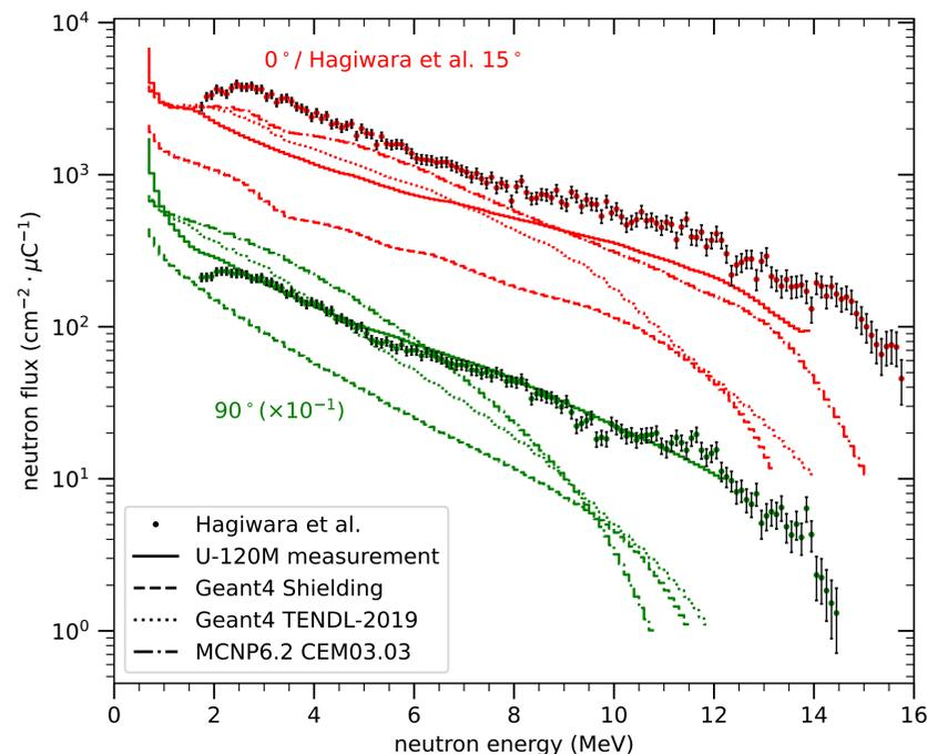
Fig. 3: Comparison of neutron spectra in different angles with EXFOR database (Hagiwara et al.) and calculations in various Monte Carlo codes with both models and data libraries
