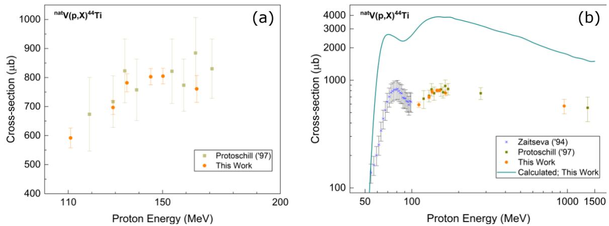
**Fig. 1:** (a) Experimental results for the  $^{44}\text{Ti}$  production from p-induced reactions, shown in comparison with previous data, and (b) comparison of the excitation function for the  $^{44}\text{Ti}$  production.
