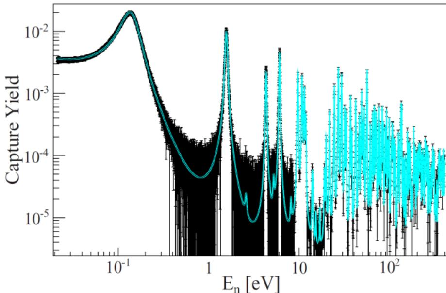
$^{176}\text{Lu}(n, \gamma)$  measured with the DANCE detector at the Los Alamos Neutron Science Center. The blue curve is a SAMMY fit.
