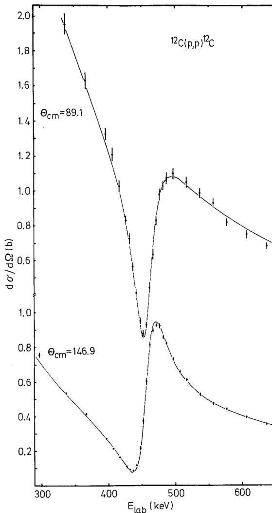
Fig. 1. Elastic scattering differential cross-section vs. the laboratory bombarding energy between 0.3 and 0.6 MeV. The solid line corresponds to the best fit parameters (Table 1) of an  $R$ -matrix analysis
